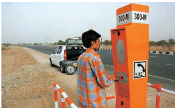
Fig. 7.10 : Emergency call box on NH-48
