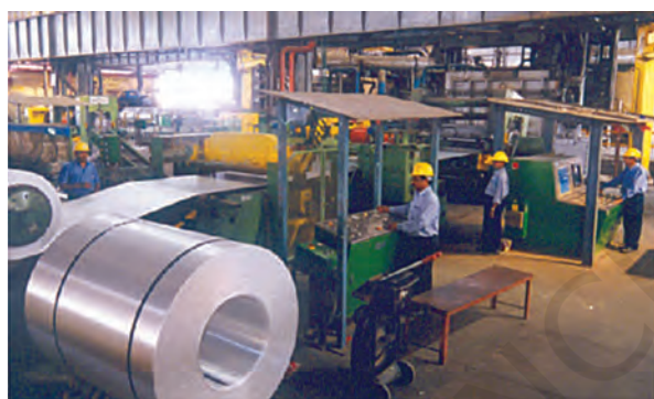
Fig. 6.3: Strip casting mill at smelter of NALCO
