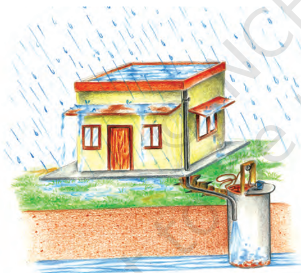
(b) Recharge through Abandoned Dugwell
