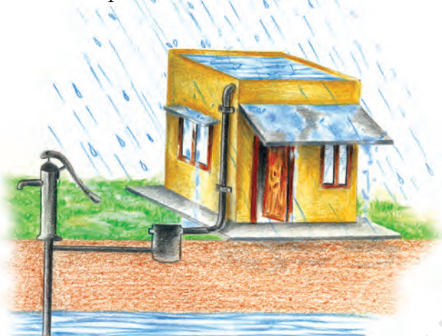
(a) Recharge through Hand Pump
